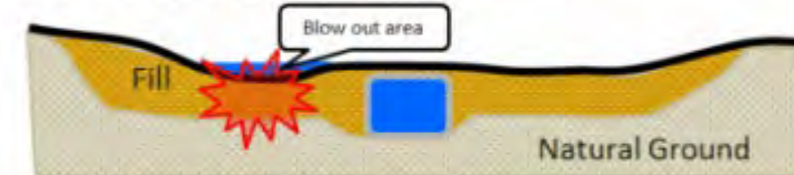
Figure 2. Typical Blow-out at low spot in road
