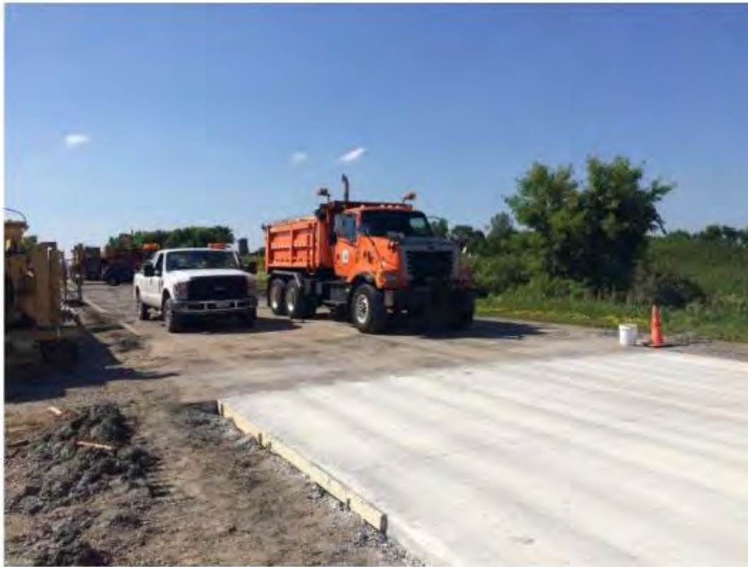
4,000 lb axle vs 14,000 lb axle loads (1 st Cell @ 3hrs)
