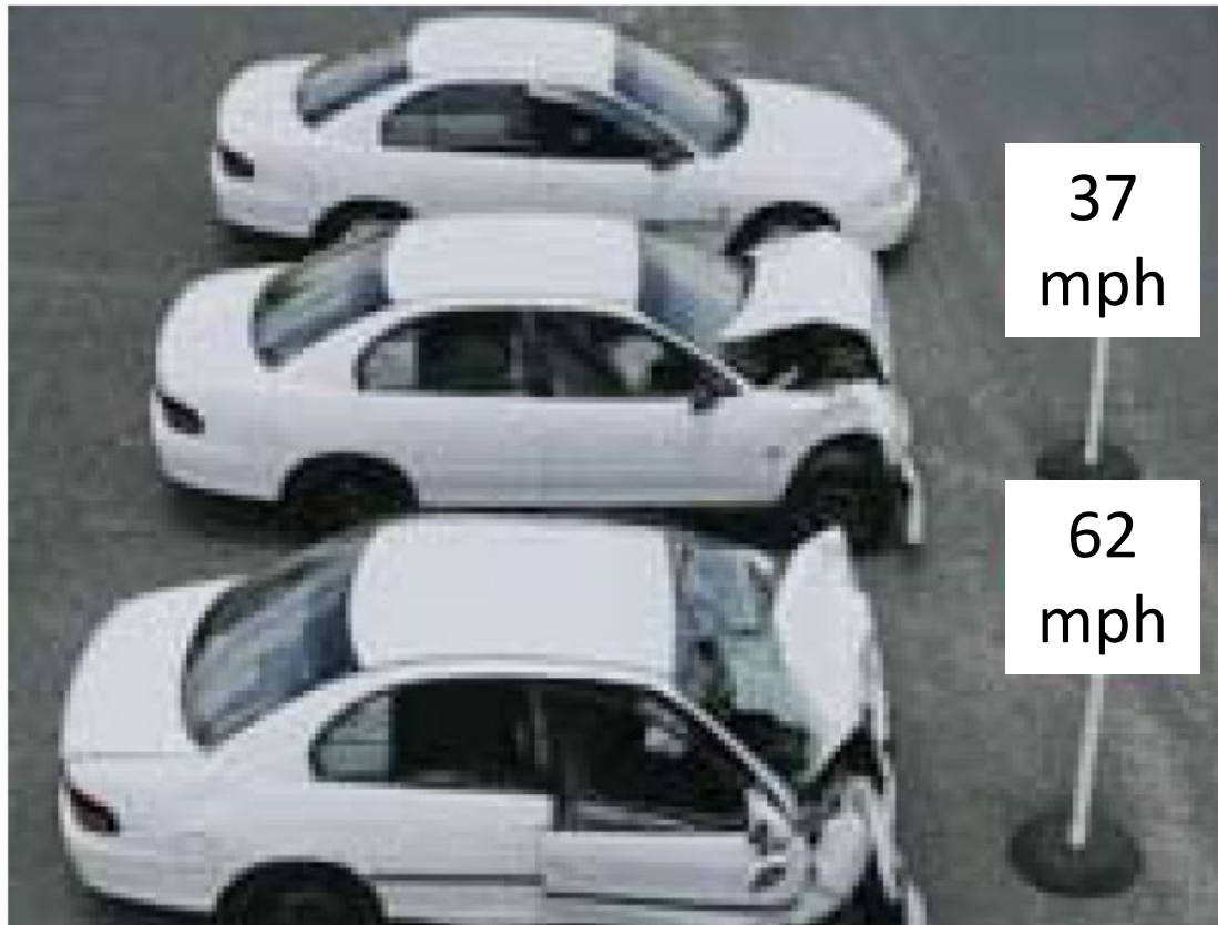
Figure 4.5: Difference in deformation striking a solid object at 60 km/h and 100 km/h
