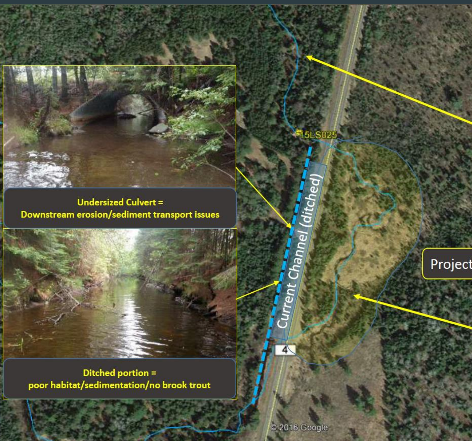
¼ mile of natural channel disconnected from Humphrey Ck via roadside ditch
