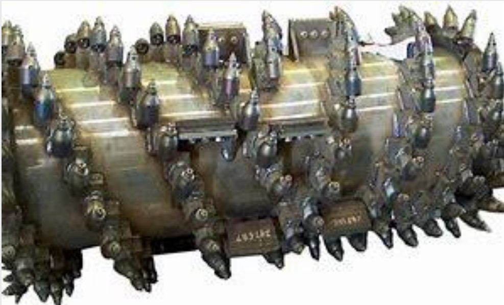
Traditional Milling Head Teeth spaced about 0.625 inches apart
