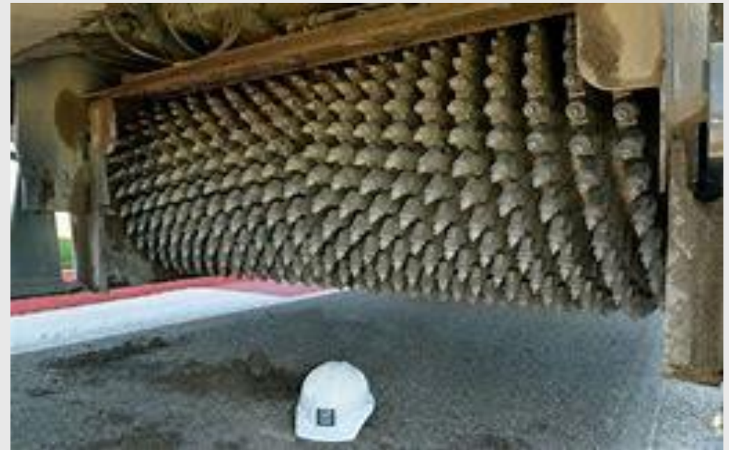
Micromilling Head Teeth spaced 0.200 inches apart
