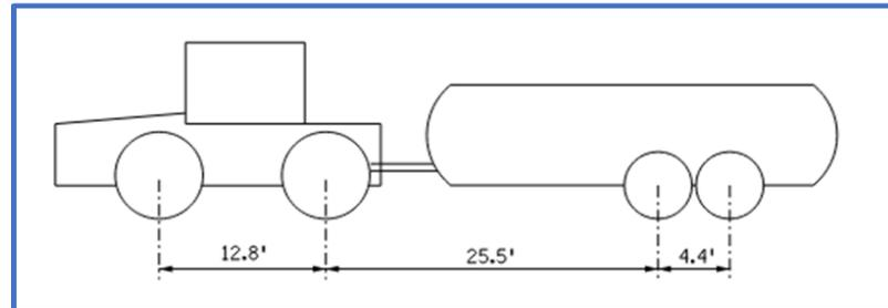
Footprint and Schematic Elevation View of New Holland T8040 tractor towing a Better-Bilt 4950 manure spreader. Total weight of vehicle is 87,754 LB.
