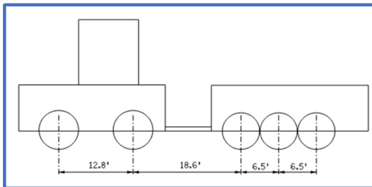
Footprint and Schematic Elevation View of John Deere 9620 tractor pulling a Balzer 1500 Grain Cart. Total weight of vehicle is 143,679 LB.
