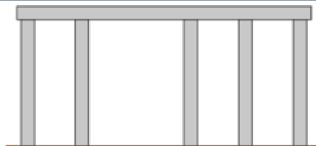
Figure 6.2 Assume deteriorated pile is ineffective.
